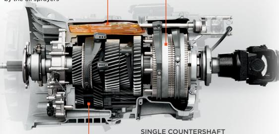
A single countershaft with helical gears lowers the overall weight of the unit without compromising the durability or performance of the transmission
